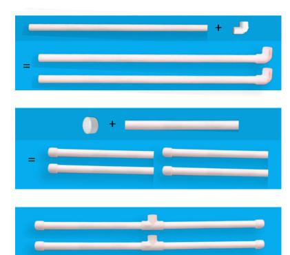
**4.** Join (1) arm piece to (1) completed foot piece. Repeat this process equaling TWO identical pieces.
