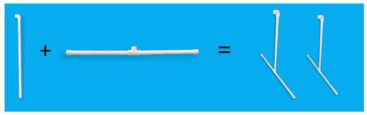
**5.** Join both ends of top bar to 90° elbow fittings on arm pieces. Your stand is complete.
